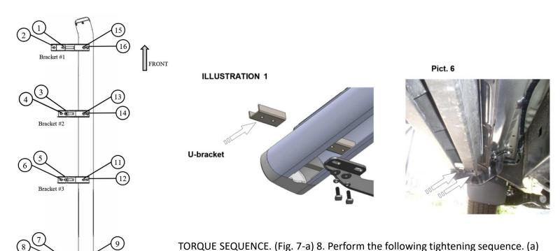
Torque all body fasteners to 16.3 Lbf-ft (22.1 Nm). (b) Torque all board fastener to 16.3 Lbf-ft (22.1 Nm).
